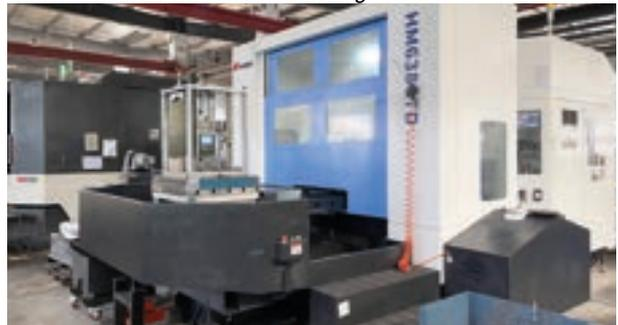
Dentatrice CNC - *CNC gear cutting machine*
