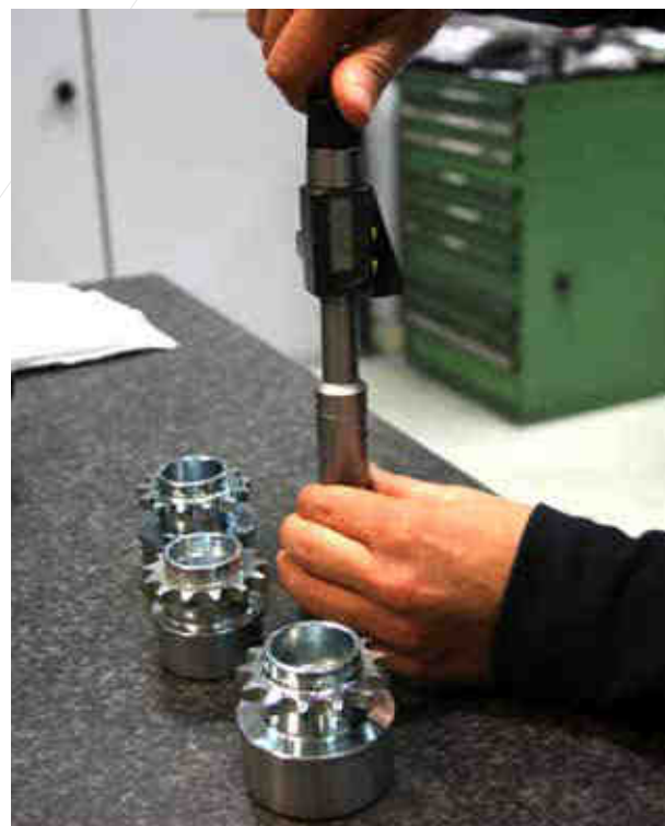
Controllo tolleranza testate - Diameter tolerance check (roller ends)
